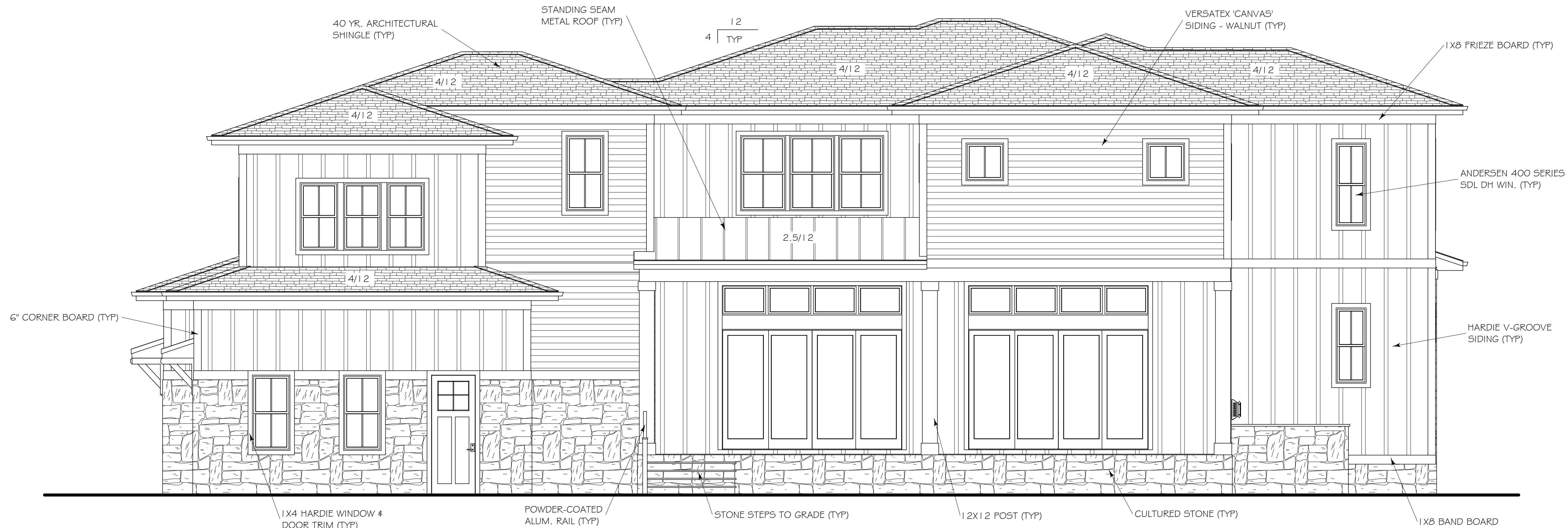
A REAR ELEVATION SCALE: 1/4" = 1'-0"
